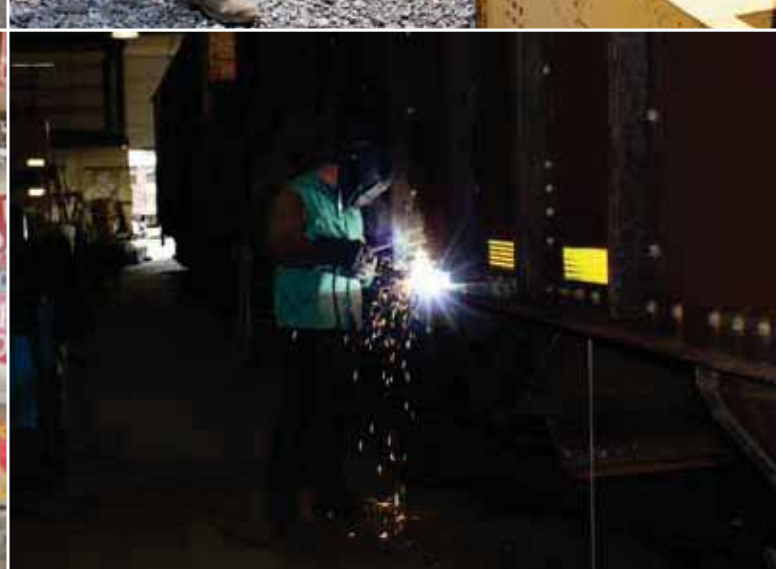
Jim Somers welding an RBMN open top hopper car.
