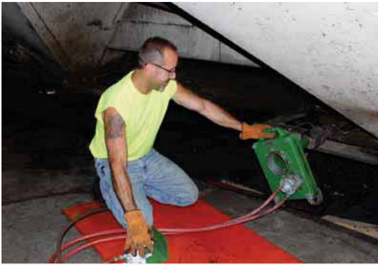
John Dubick opening a covered hopper gate with a power door opener.
