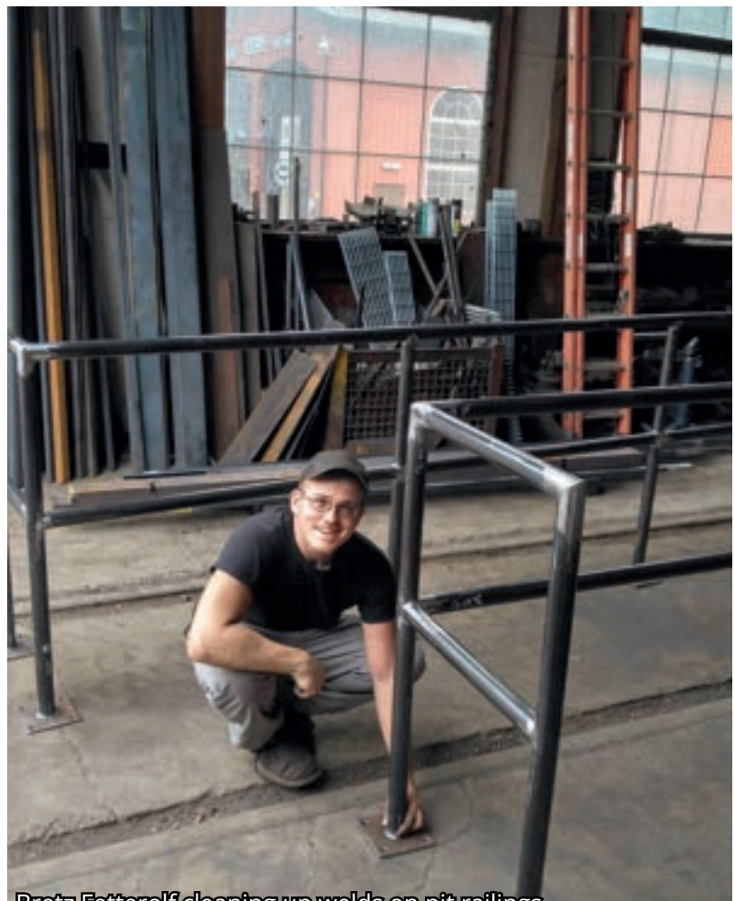
Bretz Fetterolf cleaning up welds on pit railings.
