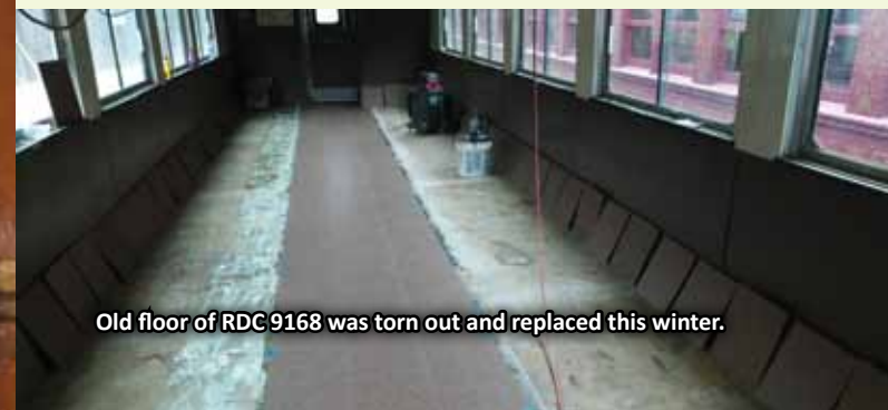
Interior of RDC 9168 half way through floor installation.
