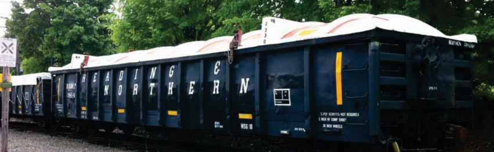
Side view of RBMN 3814 with the new hard cover attached. The hard cover was added when the car was in Canada, and replaces the tarps that were previously used on these cars. A car that is equipped with one of the single-use tarps is visible on the left side of the photo.
