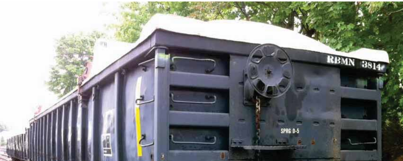
End view of the RBMN 3814 with the new hard cover attached. The RBMN car shop modified these cars to accommodate the use of the hard covers, and eliminate the need for single-use tarps.
